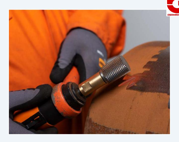
"The Safety Tools Allmet grinding tools were tested under anticipated worst case conditions – operations within explosive mixtures of propane and acetylene. It was not found possible to provoke ignition of the explosive mixtures during any of the tests performed."
